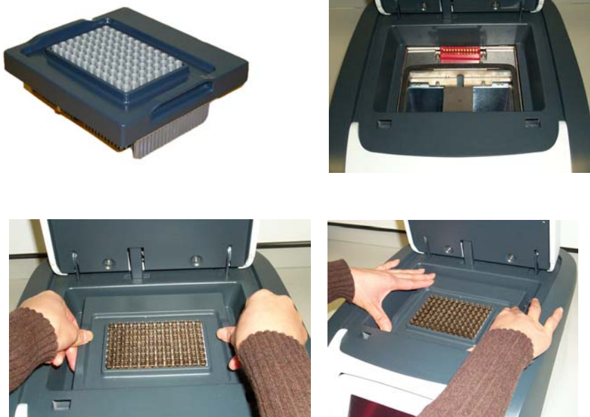
Figure 2-1: G-Storm GS1 cycler - thermal block installation
