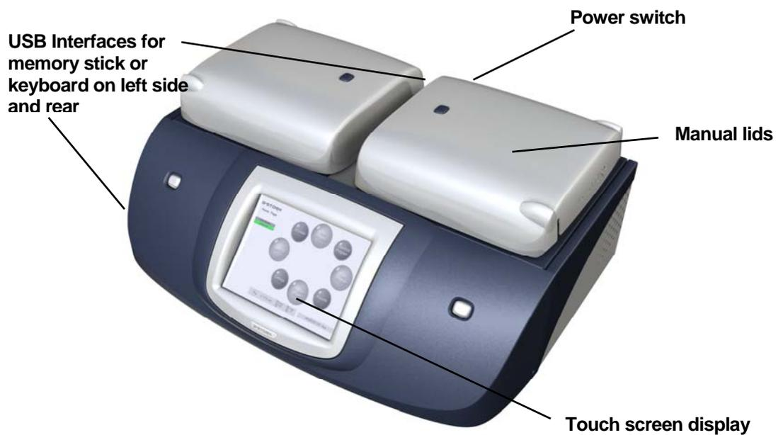
*Figure 2-2: GS2M thermal cycler (profile view)*
