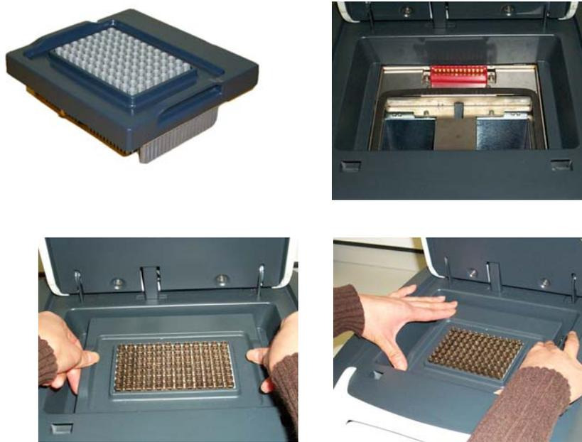
*Figure 2-1: G-Storm cycler - thermal block installation*
