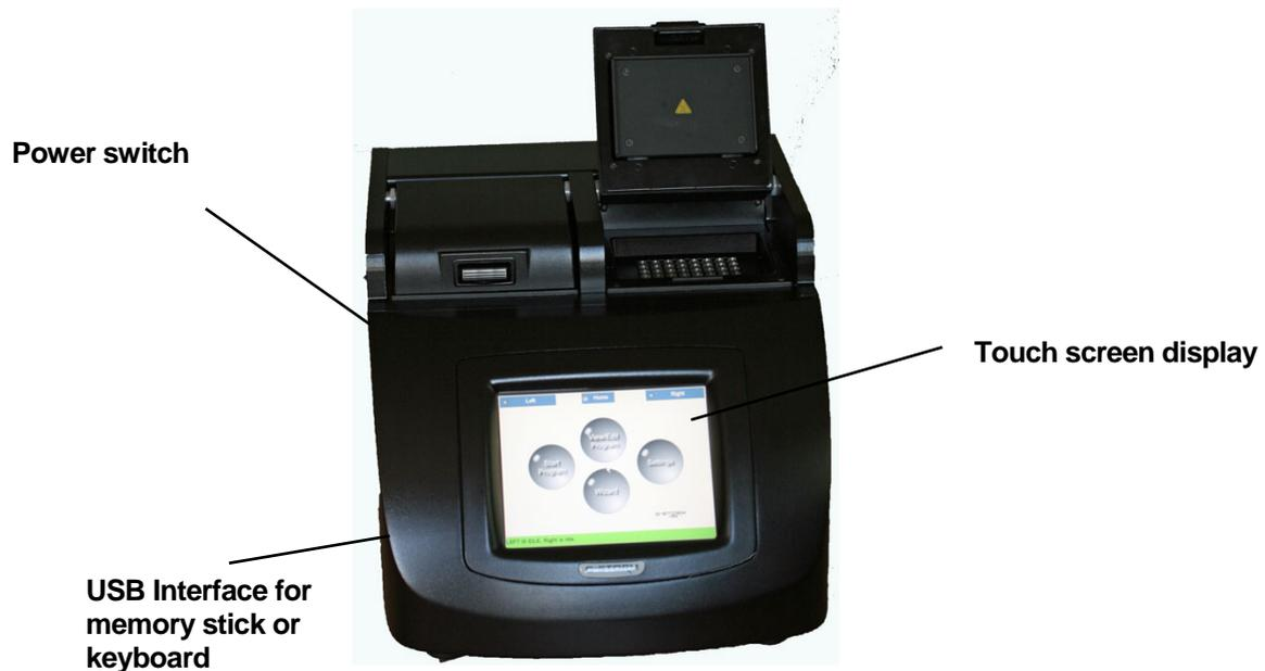
*Figure 2-1: G-Storm GS4822 thermal cycler (profile view)*
