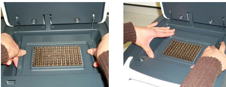
Figure 9-1: Exchanging the block
