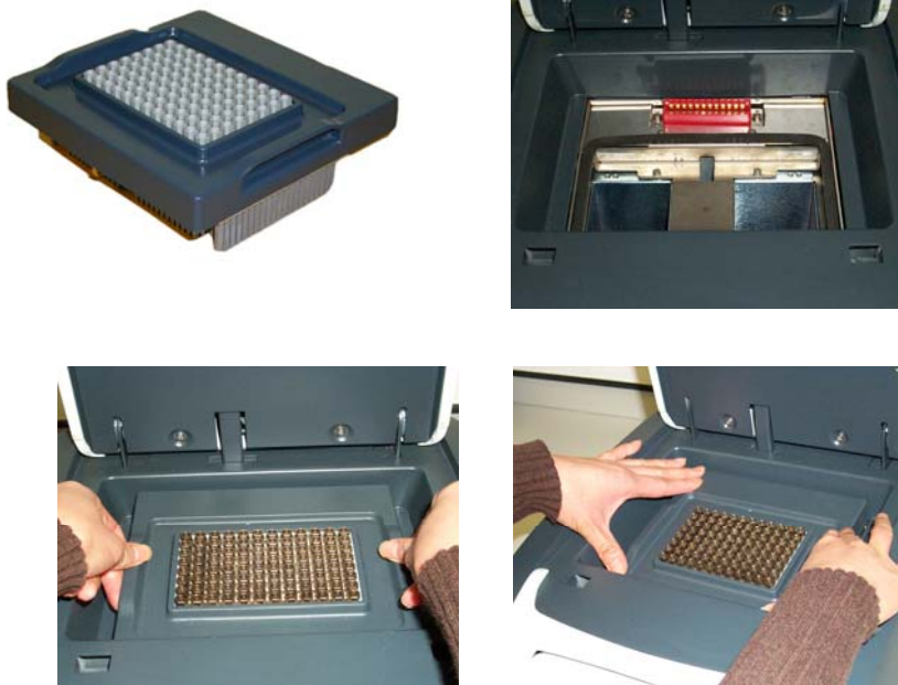
Figure 2-1: GS4M thermal cycler - thermal block installation
